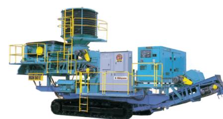
自走式土壌改良機 (Crawler-mounted soil remediation equipment)
