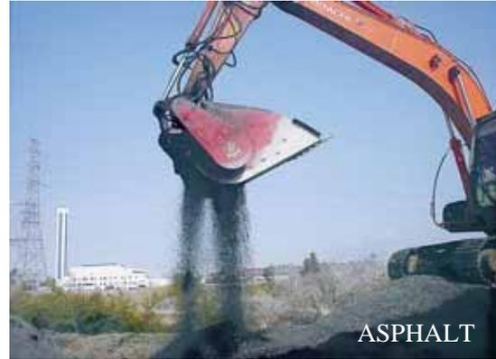
NB50FR/70FR produce materials of cubical form and can process other materials such as concrete blocks, bricks, roof tiles, friable stones, shells, slag, etc. It can be used also for mixing composts and fertilizers.
